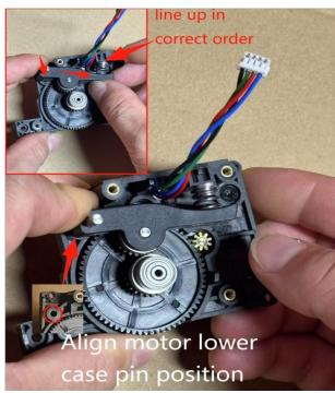
Step 2 - Installation of Extruder Upper Shell
