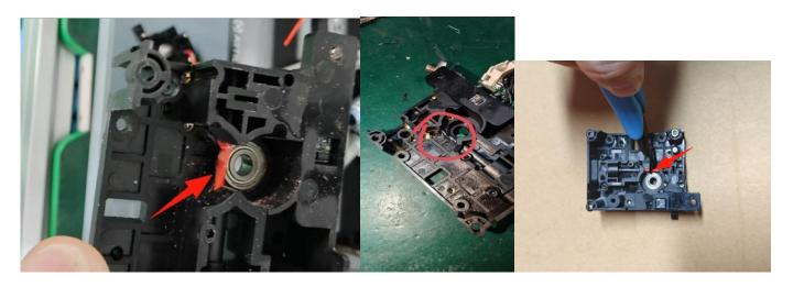
① . Remove the small cover plate (3 M2.0\*8 cylindrical head self-tapping screws) in the chamber of the extruder's upper case with a H1.5 inner hexagonal spanner and inspect the Bowden tube assembly in the chamber. (Remarks: When to replace the Bowden tube assembly - when jamming the tube (PTFE tube), it is easy to dislodge by pulling with slight force and can be replaced.)
