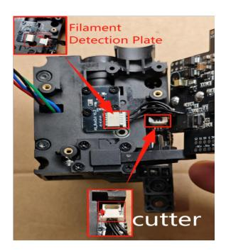
② . Install the extruder motor wire terminal into the extruder circuit board motor holder. Use PH1 Phillips screwdriver to lock the extruder circuit board to fix 4 M2.5\*5 Phillips flat head screws. And turn the extruder assembly to the left side, check the cutter and break material lead must avoid the cutter handle position. To prevent the cutter cut material function failure.
