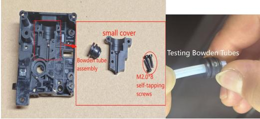
② . Planing material - Clean the extruder chamber with a soft bristle brush. And use a small cotton swab to stick a little grease on the extruder motor pinion.
