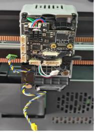
② Remove the 4 fixing screws (3 M2.5\*10 flat head screws and 1 M2.5\*8 flat head screw) on the extruder with the H1.5 hexagonal spanner. Remove the extruder assembly.
