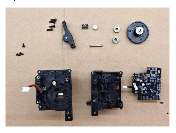
① .Install bearings on both ends of the large gear shaft and install it in the extruded lower case motor gear end position.
