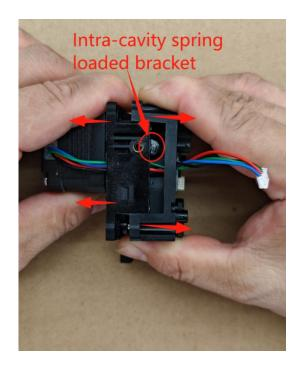
Step 7 - Extruder cavity cleaning
