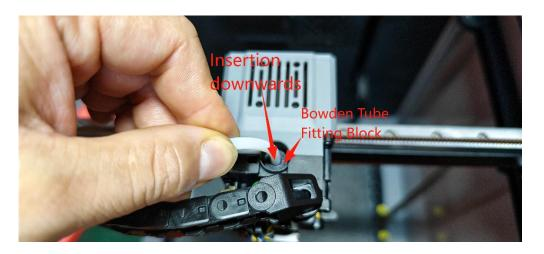
Step 6-Installing the Hot End Assembly
