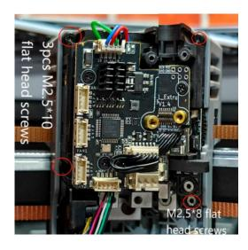
Step 5 - Removing the Extruder Circuit Board
