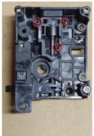
② .Assemble the extruder shell - first, put the lower shell motor leads into the upper shell motor outlet, and butt the upper and lower shells to install the compression. Use H1.5 hexagonal spanner to lock the fixing screws (4 M2.0 \* 8 flat head self-tapping screws) and the left side of the tightening nail screws to screw the surface of the extruder shell can be flat. As shown in the picture:
