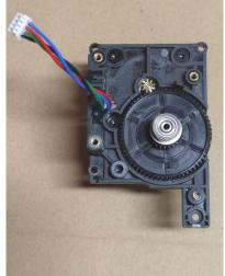
② .Right hand fingers pinch (handle assembly & compression spring, spring holder end) together and snap into place to install until major gear shaft pinion is aligned. Left fingers pinch the handle pin end to align the motor lower case pin position. Right fingers press the spring bracket to align the tightening nail screw position loosely, press the handle pin to the lower case lock fixed.
