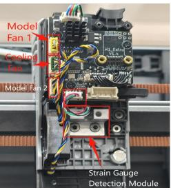
Step 5 - Install Extruder Cable Retaining Screws
