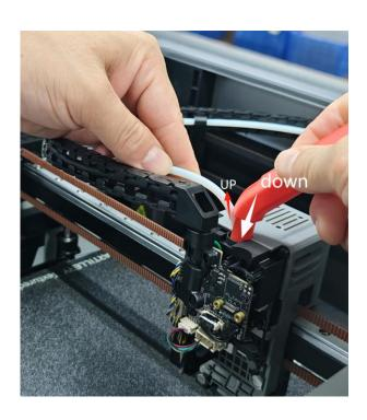
Step 4 - Remove Extruder Set Screws
