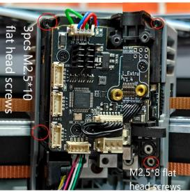
②. Plug the hot-end cooling fan and the rear-end drum fan 1, and the strain gauge detection module terminals correspondingly to the extruded circuit board holders.
