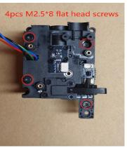
① ① . Separate the upper and lower extruder shells slowly in the opposite direction of the arrow in the figure. (Note: Extruder handles, springs and spring retaining brackets in the extruder chamber should not be dropped or lost)
